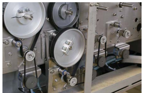
Image 6 Wachendorff encoders measure with millimetre accuracy the distance the fish have travelled in the machine.
