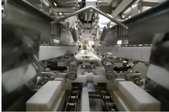
Image 7 A view of the inside of the machine, showing in the foreground where initially the length is measured. In the background the knives can be seen, which are waiting to remove the head, fins, skin and bones.
