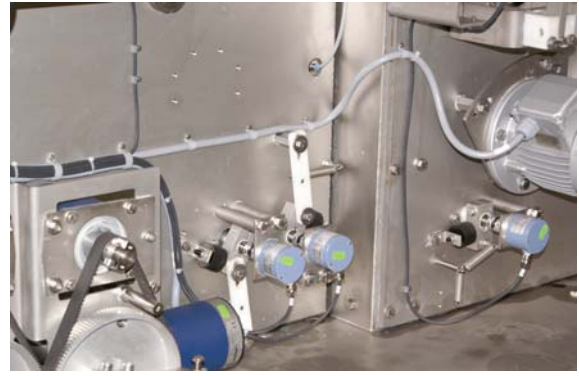
Image 4 A wheel, mounted via a spring arm, measures - with the help of an encoder from Wachendorff - the length of each individual fish and then transmits the values on to the controller for the cutter motor.
