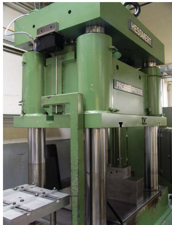
Image 2 A draw-wire system with an encoder on each hydraulic ram allows for precise determination of the position
