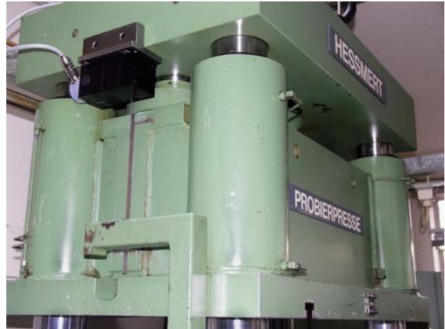
Image 5 Elderly hydraulic press with the latest control technology
